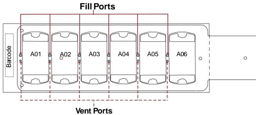
Figure 5: HX6 Mixer and Slide for a CGX-6 Array
