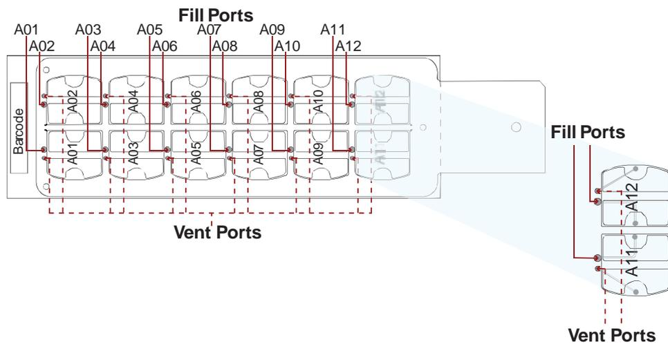
Figure 6: HX12 Mixer and Slide for a CGX-12 Array
