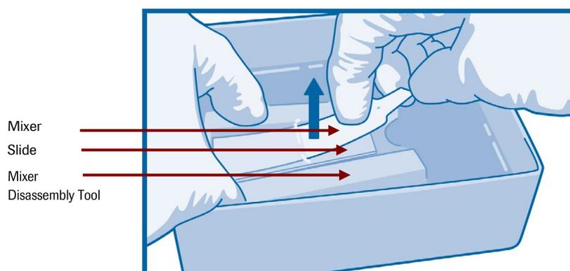
**Figure 7: Using the Mixer Disassembly Tool to Remove a Slide from a Mixer**
