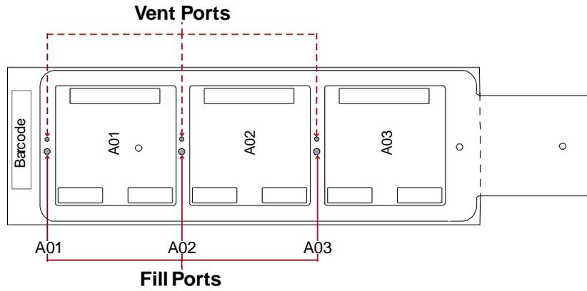
Figure 4: HX3 Mixer and Slide for a CGX-3 Array
