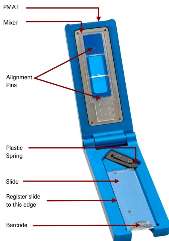
**Figure 3: PMAT with HX3 Mixer and Slide.** For photographic purposes only, blue coloring was used to show the location of the mixer's hybridization chambers. The hybridization chambers of the mixer you receive will not be blue.
