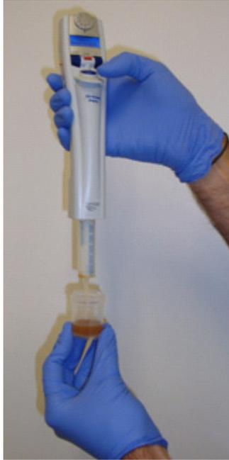
**Figure 12** Filling the 10-mL Combitip Plus tip with the aqueous phase and bead mixture using the Xstream pipettor.
